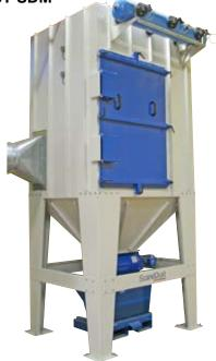
ScandDust SDM is a modular designed dust collector with rectangular filterhousing. Smallest module has four filter cartridges and largets module has 12 filter cartridges. SDM is always connected to an external fan.
