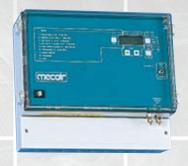
The internal differential pressure sensor register the progress of the pressuredrop over the filter. When it exceeds the set value the cleaning sequense is started automatically.
